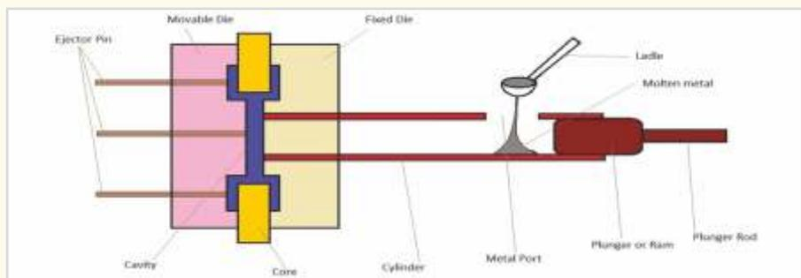
A high-pressure die casting machine has many moving parts that require lubrication and some of these are shown in the diagram below.
