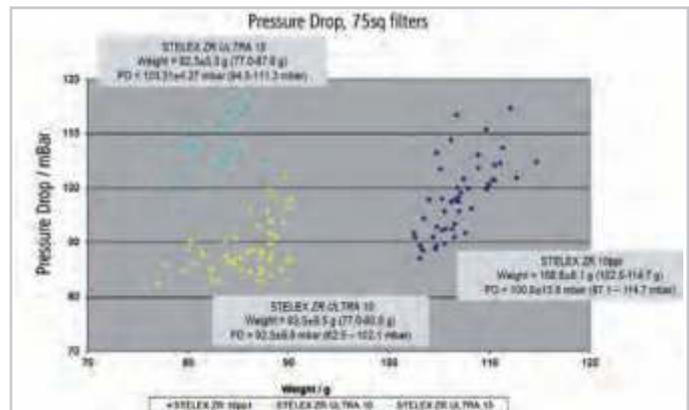
The results show that pressure drop associated with STELEX ZR ULTRA 10 is 9% lower (better) than standard STELEX ZR 10ppi, despite the STELEX ZR ULTRA 10 porosity being purposefully finer to deliver a higher filtration efficiency. The pressure drop associated with
