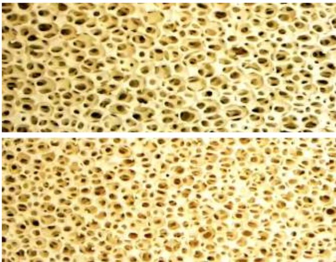
The intention is that STELEX ZR ULTRA 10 will provide a filter that consistently primes and provides reproducible performance in terms of metal flow rate and capacity before filter blockage. STELEX ZR ULTRA 15 will provide enhanced filtration efficiency where required and will be particularly well suited to high specification, high integrity, high alloy casting applications.
