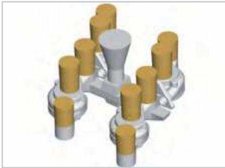
On a specific casting the foundry was using 75x75x25mm 10ppi zirconia foam filters but was still suffering a reject rate of over 2% for a combination of slag defects and particles of filter, due to filter friability. Previously the foundry had tried to use finer filters but these had not been accepted as they introduced metal pouring and flow associated problems. The foundry initially assessed 400 units of STELEX ZR ULTRA 15, the results of the experiment are shown in the table.
