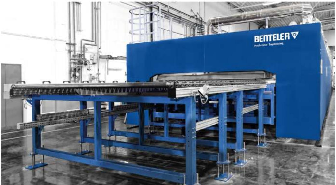
Figure 1 : Example of Roller Furnace for Hot Stamping Line [Source : BENTELER Automotive]
