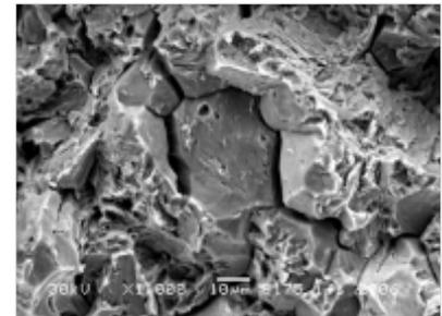
**Figure 5 :** Example of Hydrogen Embrittlement Crack
