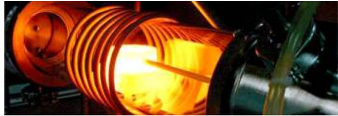
a critical cooling rate. The resultant structure known as ‘Martensite’ is hard & brittle phase with a BCT (body centre tetragonal) crystal structure, which has an elongated lattice dimension and about 4% higher volume.
