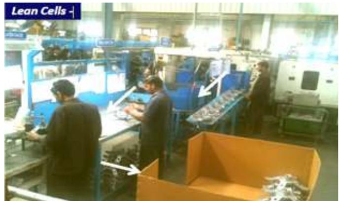
**2. O - One Piece Flow :** In order to reduce the lead time, the batch size of material flow is reduced. For example, the batch size is reduced from 1000 to 100 pieces, by using lower capacity bins. We eliminated material handling by breaking the wall between die-casting and Machining cells and using gravity conveyors. This reduced transportation of material and excess motion by 100%. We have horizontal deployment plans across all our foundries during 2016.
