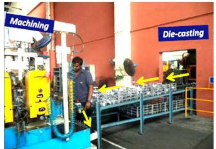
**3. P – Pull System :** We operate with a weekly pull customer model. Weekly plan is converted into a daily plan by assembly lines and pull is created. Benefits from Pull System are --Material is pulled through the
