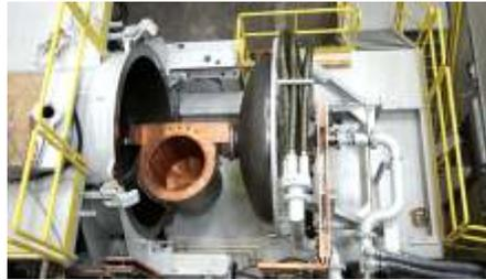
structure from overheating. Hydraulic and pneumatic systems remove air from the furnace and casting chambers, which is critical to safe handling of molten titanium.
