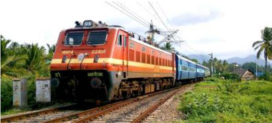
Indian Railways, which earlier used Corten steel to manufacture coaches at its Integral Coach Factory is gradually shifting towards stainless steel which is used to manufacture German Linke Hofmann Busch coaches.
