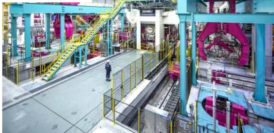
The rolling line is fully controlled and operated by the L1 and L2 automation system developed by Danieli Automation, which allows the plant to be run with just a few operators.
