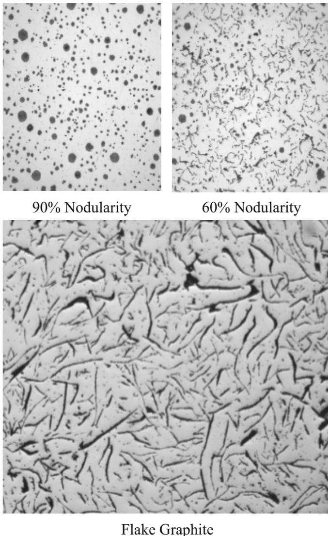
In Fig.2 Test result shows the following specification requirement 90% Form VI nodularity according to ISO945.
