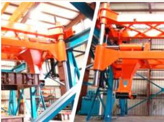
**V**ulcan Engineering recently shipped a 16 ton Gantry Style Donovan Manipulator. The unit is designed to move over a conveyor to draw the flask package, lift and move the flask to a coating area. Once there, the Rollover will rotate the flask to allow for manual coating of the mold. After coating, the rollover will move the flask to another conveyor and set the flask on
