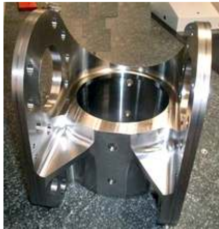
Fig. 3 - Aircraft fittings fabricated from Precipitation Hardening Stainless steels
