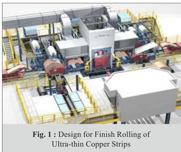
**Fig. 1 : Design for Finish Rolling of Ultra-thin Copper Strips**
