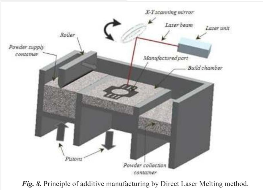
**Fig. 8.** Principle of additive manufacturing by Direct Laser Melting method.
