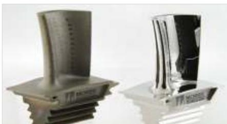
**Fig. 3.** Turbine blades laser - sintered with EOS DMLS (left) and polished with the Micro-Machining (right)
