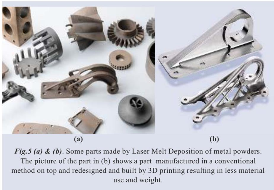
**Fig.5 (a) & (b).** Some parts made by Laser Melt Deposition of metal powders. The picture of the part in (b) shows a part manufactured in a conventional method on top and redesigned and built by 3D printing resulting in less material use and weight.
