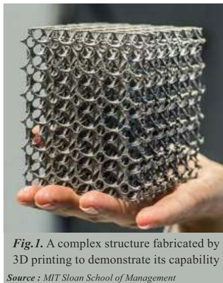
*Fig.1.* A complex structure fabricated by 3D printing to demonstrate its capability
