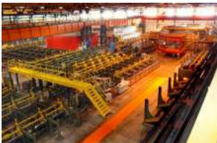
**T**MK-ARTROM based in Slatina, Romania, granted SMS group the final acceptance certificate (FAC) for the supplied tube and pipe heat treatment line. Designed for an annual capacity of 160,000 tons, the new heat treatment line will be used for the production of seamless high-strength pipes up to a wall thickness of 60 millimeters for mechanical applications as well as of special OCTG pipes (oil country tubular goods).
