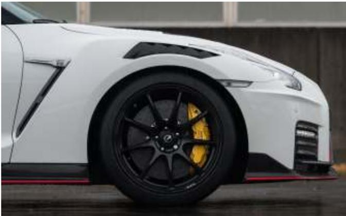
**B**rembo, together with Nissan technicians, have engineered a bespoke braking system for the 2020 Nissan GT-R NISMO and Track Edition. Brembo's one-piece, six-piston aluminum monoblock front calipers have a more aggressive design enhancing the overall look of the GT-R.
