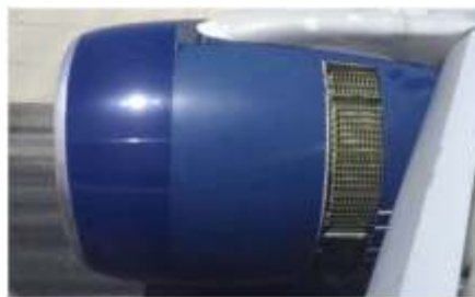
Fig. 04. Thrust reverser cascade casting made of Magnesium alloy
