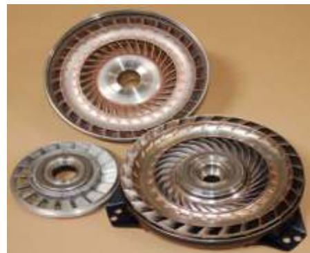
Fig. 06 Impellers brazed with Gold fillers
