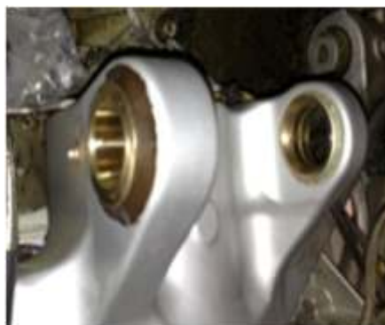
Fig. 07 Aircraft Landing gear with Bronze Bushing
