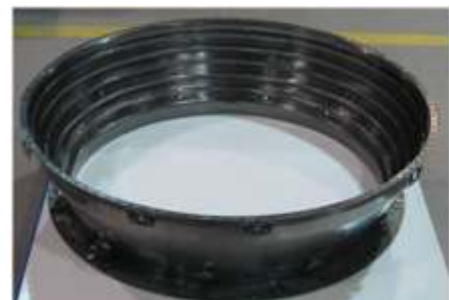
Fig. 2 . Low Pressure Turbine ( LPT ) Case of an Aeroengine made from Nickel alloy Inconel 718
