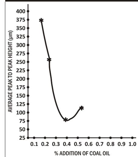
**Graph 5.3 : Average Absolute Height (µm) vs % Addition of Coal Oil**
