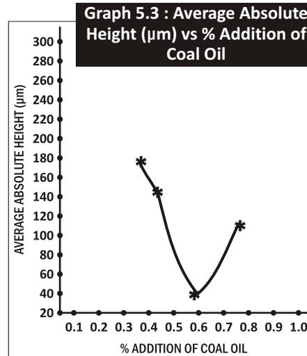
values with 0.4% addition of coal oil are RMS average = 161.6m, Average peak to peak height = 252.5m and Average absolute height = 144m. The values decreases to RMS average = 39m, average peak to peak ht = 78.13m and average absolute height = 42.4m when 0.6% coal oil gives better surface finish than 0.4% addition of coal oil. From the Table-1 and Table-2, it was found that because of this adequate quality control of the components that were taken for study, the rejection rate has decreased from
