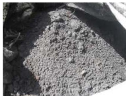
With proper Smelting process Soda iron slag is produced which is chemically stable in nature. Other type of Slag produced during the smelting process is Ferro Silicate Slag which again is chemically stable.
