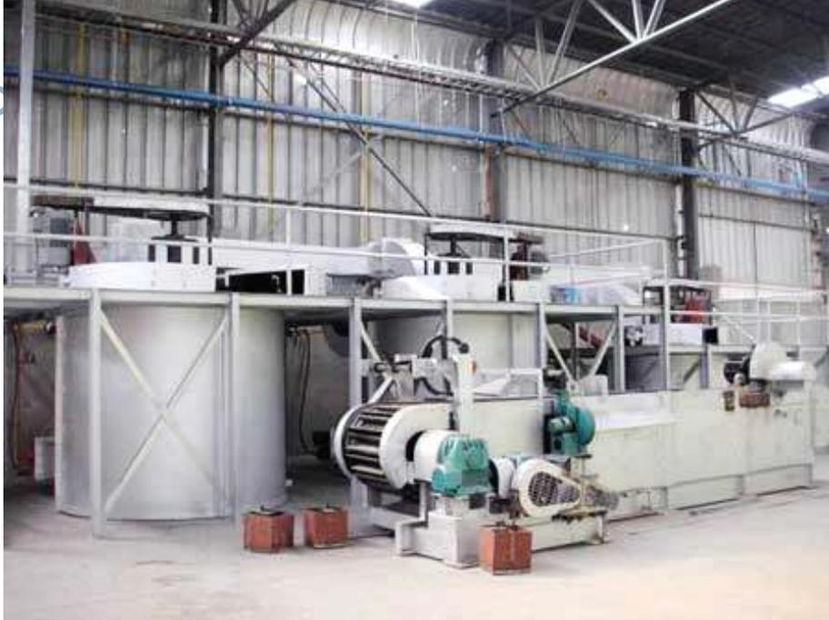
system the batteries are crushed and the crushed contents of the batteries are washed and separated into metallics, lead paste and polypropylene. In india most of the recycling units break and separate the components manually due to economic compulsions. But many are planing to put the crushers/breakers to make the breaking system cleaner and faster.
