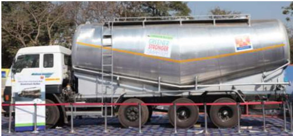
Hindalco put on display an Aluminium Bulker – the indigenously manufactured dry bulk carrier in India, demonstrating the lifecycle cost advantage offered by aluminium over other materials due to light weighting in terms of extra payload carrying capability, lower ownership cost, faster payback period, more revenue generation, low fuel consumption, reduced greenhouse gas emissions and longer life.
