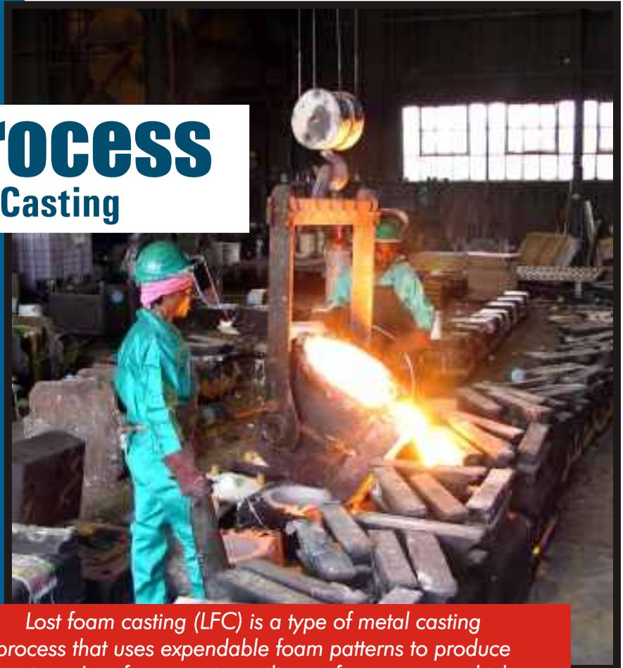
*Lost foam casting (LFC) is a type of metal casting process that uses expendable foam patterns to produce castings. Lost foam casting utilises a foam pattern which remains in the mould during metal pouring. The foam pattern is replaced by molten metal, producing the casting. With LFC, the foam pattern is moulded from polystyrene beads. LFC is differentiated from the full mould method by the use of unbonded sand as opposed to bonded sand.*
