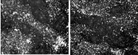
Figure-8 : (a) Microscopic Images Under 50X Magnifications for the Improved Casting Surface and (b) Showing the Reduction of Surface Cavities
