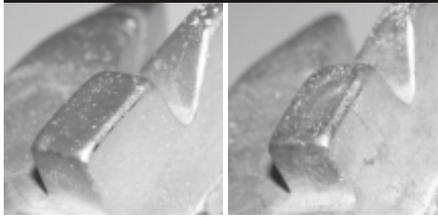
Figure-10 : Comparison of Parting Line Area and Surface Finish Improvement After Gypsum Addition, (left Side) and before Improvement (Right Side)
