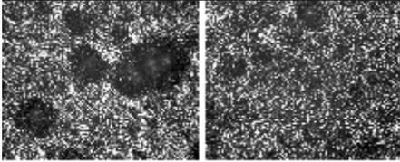
Figure-7 : Casting Microstructure After Gypsum Addition Magnified At 50x
