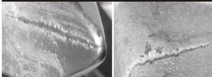
Figure-10 shown above focus the parting line area in the casting. The left side of the picture indicates the improvement done on casting after gypsum addition, whereas, the picture displayed at the right side indicates the flash formation on the casting parting line area. Flash formation on the parting line area will be followed by extra removal process.
