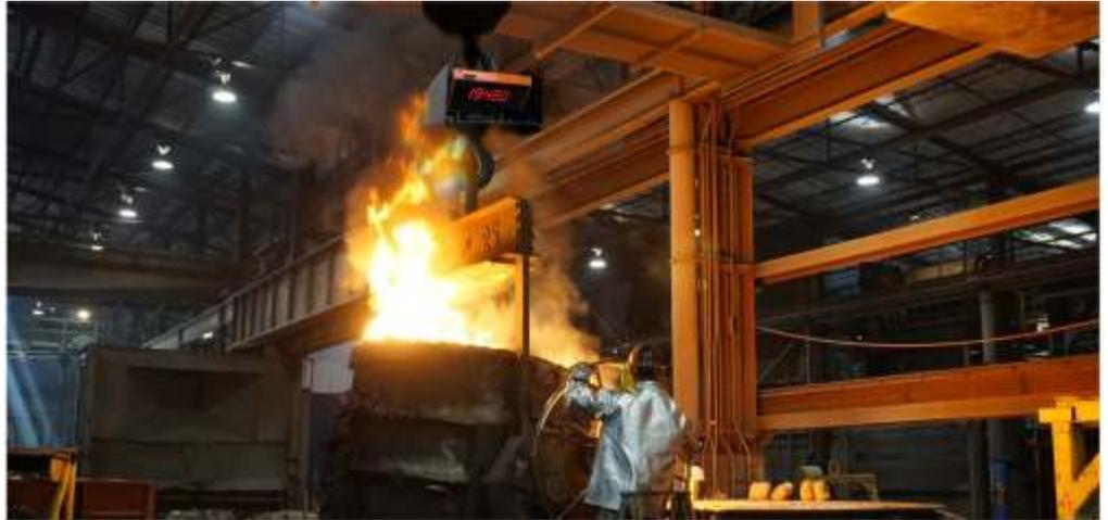
and develops therefore special solutions like the heat protected KGW crane scale. Engineered for foundry needs – heat protected to weigh material up to 1,600°C safe and precise.
