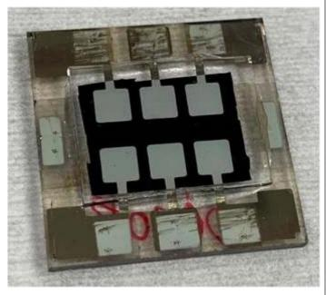
Researchers were able to fabricate this perovskite solar cell that overcomes problems with stability. Image Credit: National Renewable Energy Laboratory (NREL).
