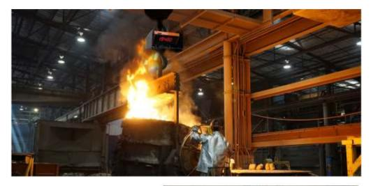
and develops therefore special solutions like the heat protected KGW crane scale. Engineered for foundry needs – heat protected to weigh material up to 1,600°C safe and precise.
