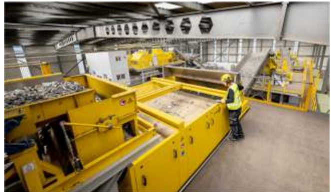
The STEINERT EddyC eddy current separator recovers non-ferrous metals (in the forefront). STEINERT KSS sensor sorting machines separate into aluminium, brass, copper and zinc.
