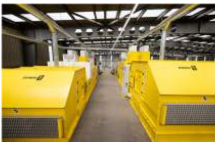
The X-ray transmission generates the purest aluminium products (on right), the STEINERT KSS XF | CLI with X-ray fluorescence delivers the purest copper, brass and zinc products.
