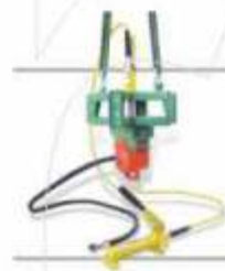
FURNACE LINING VIBRATOR
