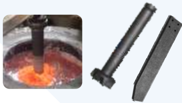
Degassing Rotor & Baffle Plate
