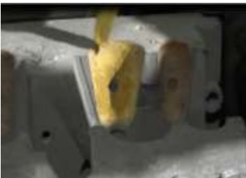
Coating applied on the riser
