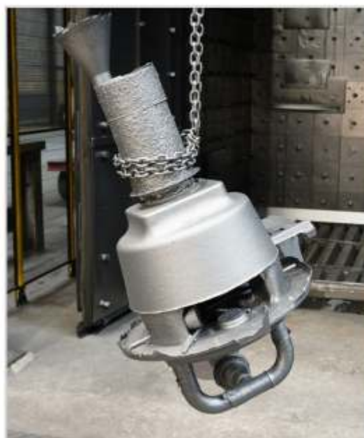
Figure 12. The planet carrier produced with STELEX Optiflow3D after shake-out
