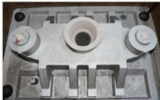
Figure 9. The STELEX Optiflow3D filter on the pattern plate
