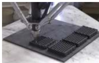
Figure 2. Research into the production of extruded 3D printed filters
