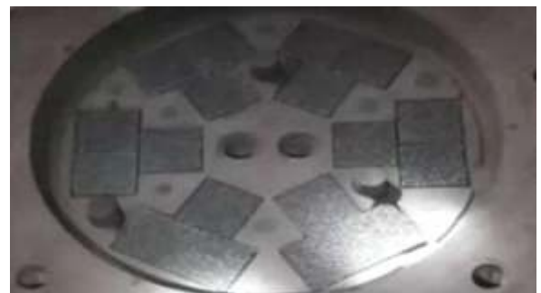
Figure 7. 18 pieces STELEX PrO 150x150x30/10 ppi applied to an iron windmill rotor hub
