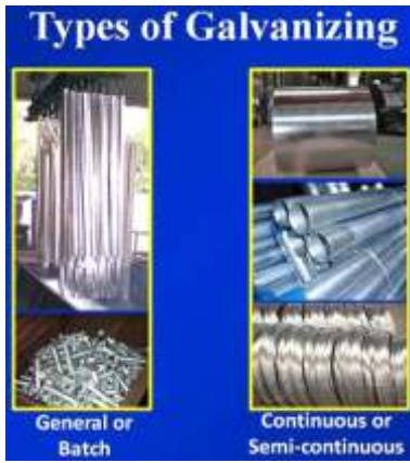
(Fig-5) Even among hot dip galvanizing, there are two types: batch galvanizing and continuous galvanizing
