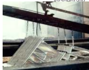
(Fig-3) A factory controlled metallurgical reaction of zinc and steel that provides "barrier" and "sacrificial protection" to steel
