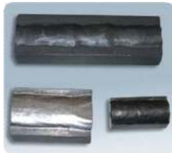
Figure 1: Examples of typical weld seam test samples.
