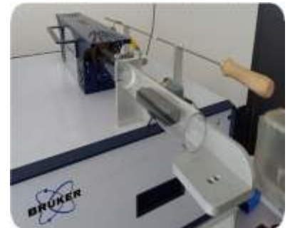
Figure 2: G4 PHOENIX Sample resting at the front part of the quartz tube, ready to be inserted.
