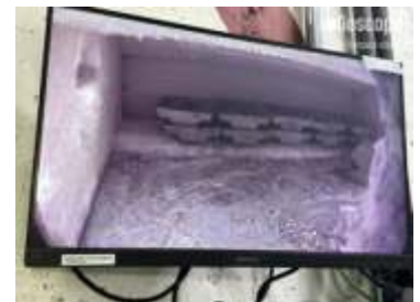
Figure 2: Real time melt cycle feedback for operators in the safety of the control room
