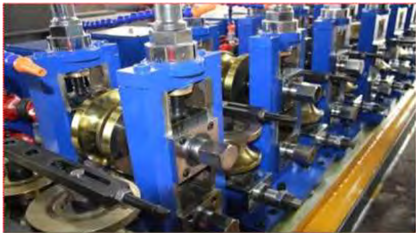
Fig.3: Precision Tube Rolling Mill
